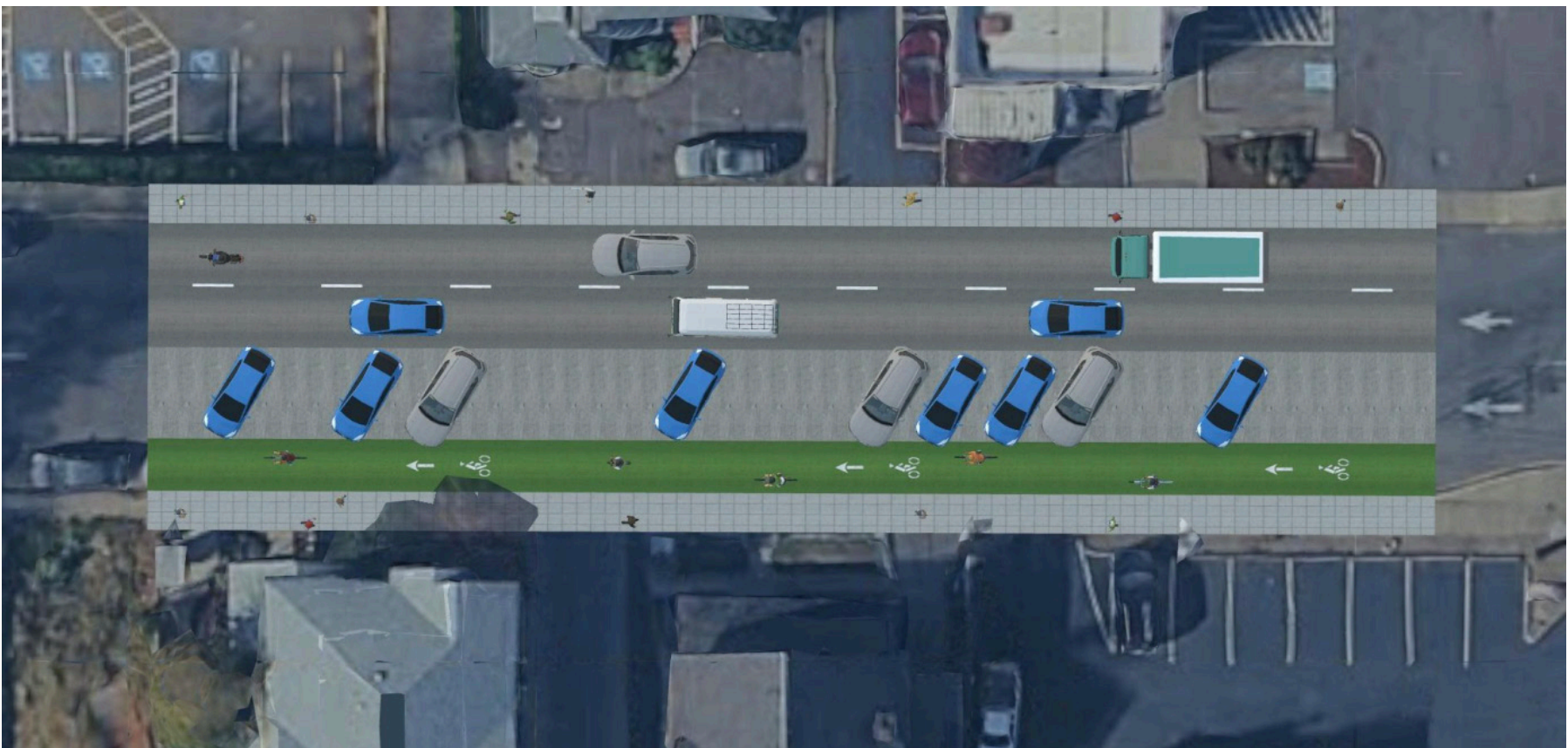
Figure 19: A Patterson Redesign showcasing an enlarged bike lane separated from travel lanes by angled parking.
