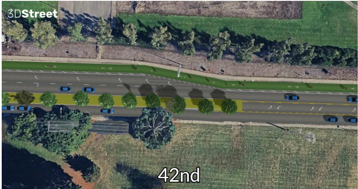
Figure 17: This redesign of 42nd Street adds a protected bikeway, a barrier protecting bikes from right turns, and room for additional green space.
