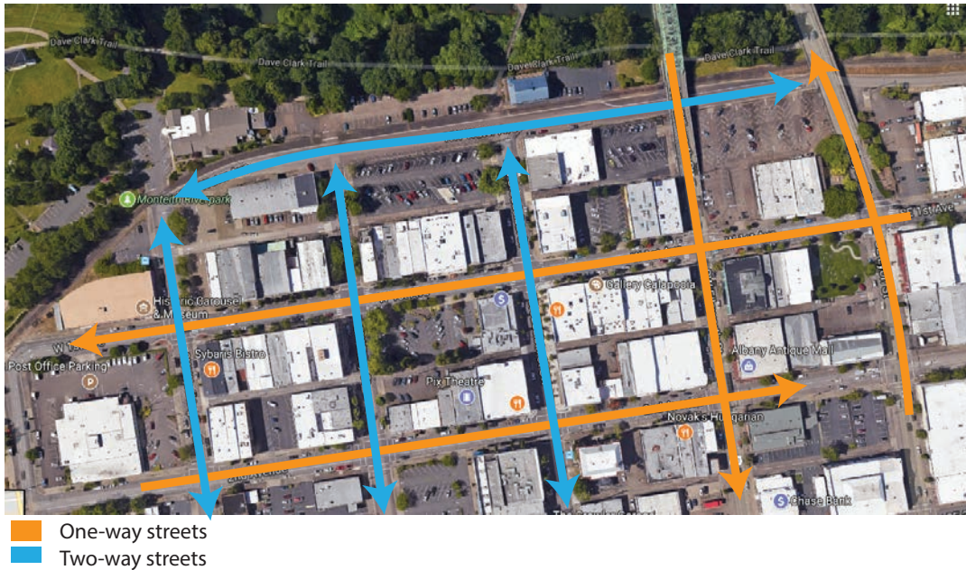
Figure 12: Current street traffic flow and parking conditions of downtown Albany.
