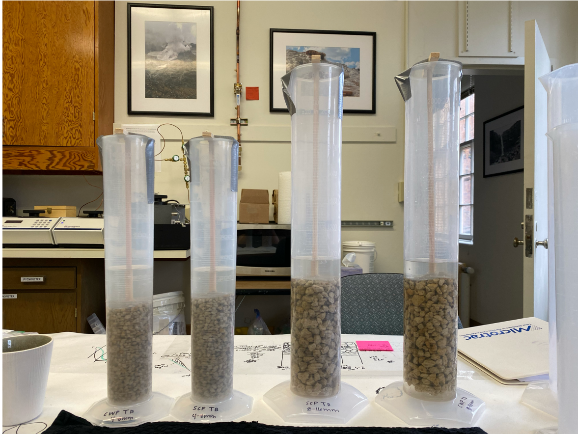
Figure 15: Graduated cylinders containing graywater and pumice clasts during still-water graduated cylinder experiments
