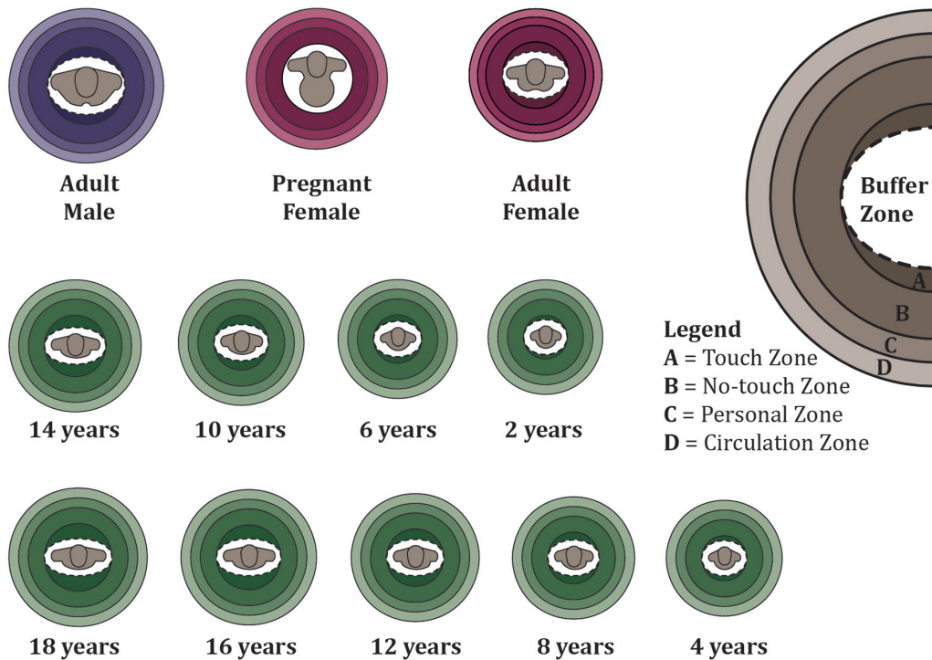
Fig. 33. Diagram of human spatial perception zones at the ages with significant changes in body size. Drawn by Jobie Hill.
