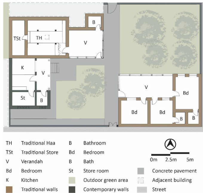
Figure 3.3. Plan of a house built in the 1950s with a subsequent contemporary addition in 2010. Adapted from Imtiaz and Rempel (2024) [78]
