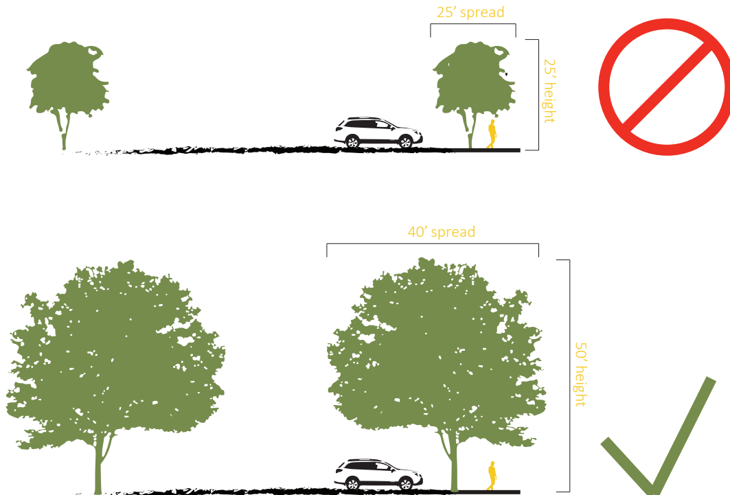
Figure 6: Small trees do not provide acceptable canopy coverage for large areas of impervious surfaces. Utilizing street trees with a larger canopy spread can collect more stormwater, mitigating runoff
