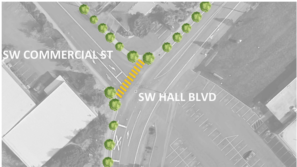
Figure 9: Adding trees to line SW Hall Boulevard provides a delineation of where crossings occur and where sidewalks lead, improving pedestrian wayfinding
