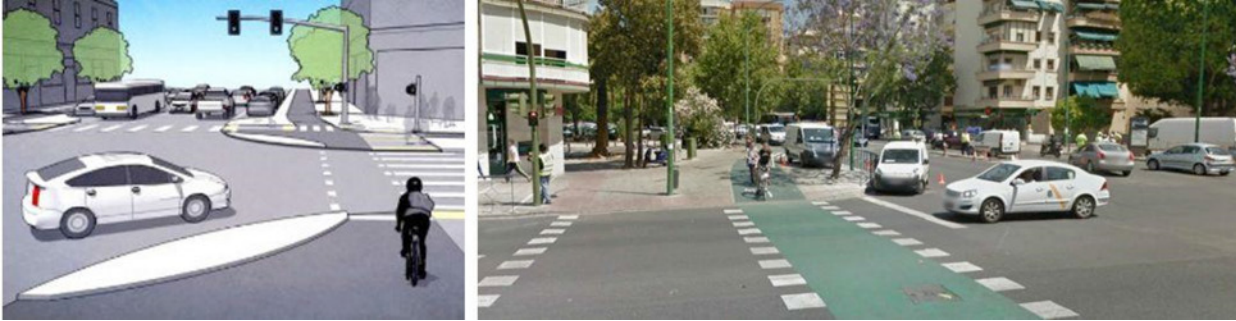
Figure 17: Bike lane setback crossing intersection (Photo credit: Sustainable Urban Design Handbook Draft by Nico Larco)
