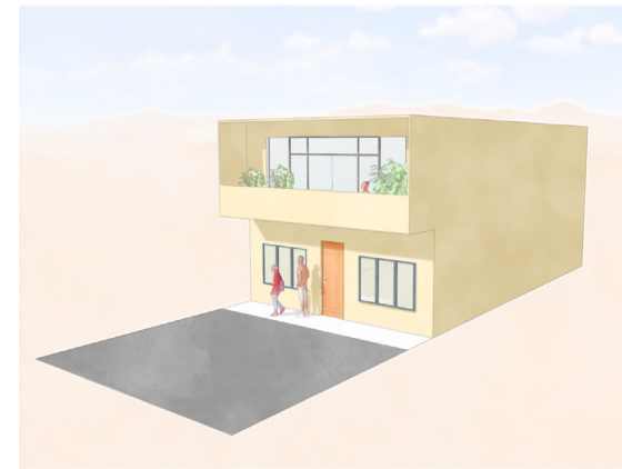
Figure 04.09. Building with Cantilever
