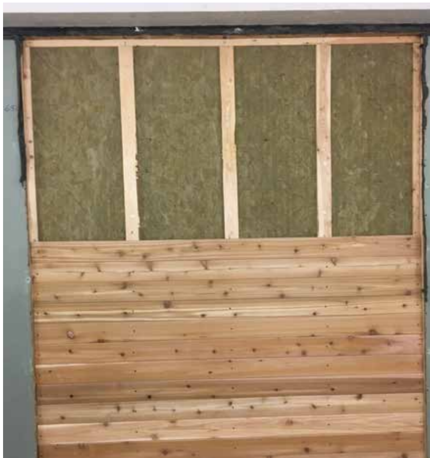
Figure 4: Specimen with membrane, insulation, and partial cedar siding
