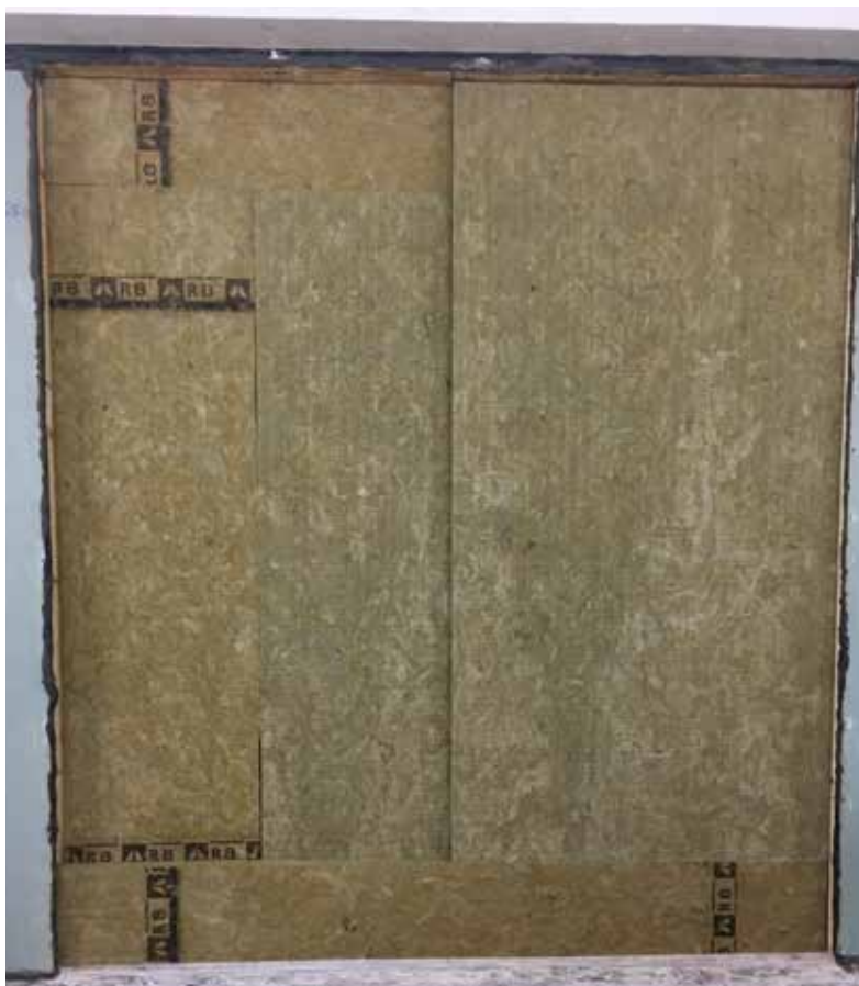
Figure 3: Specimen with membrane and insulation
