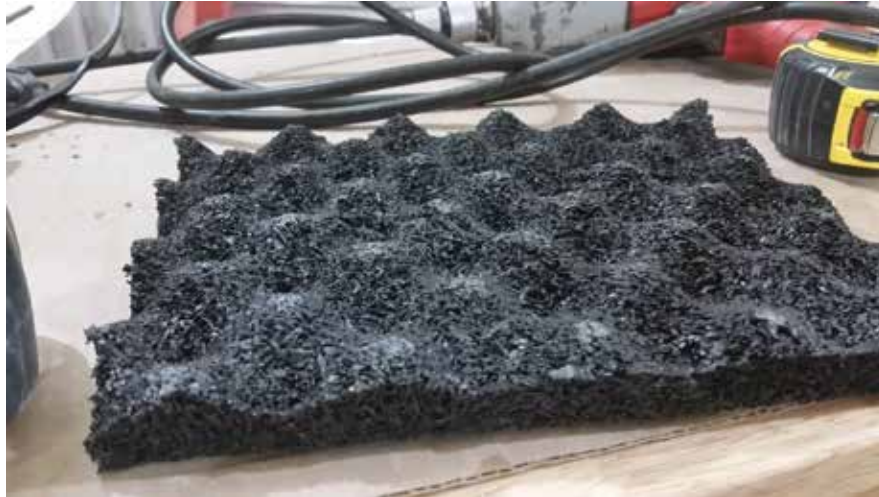
Figure 4 – Detail of bonded crumb rubber underlayment
