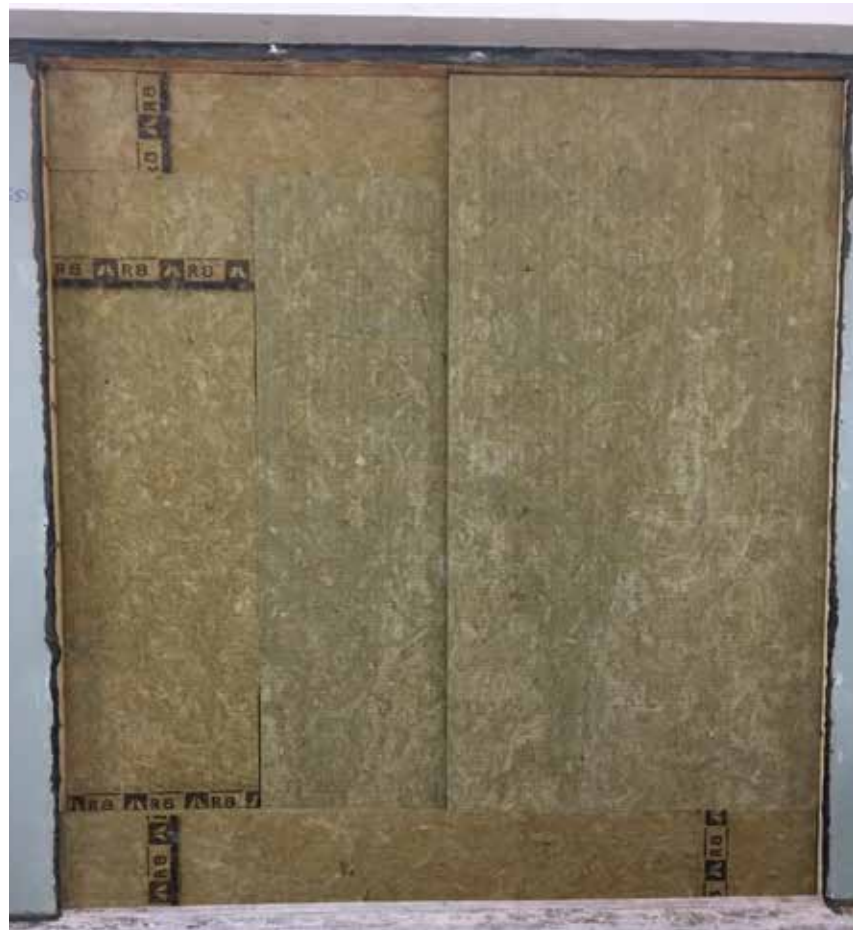
Figure 4: Specimen with membrane and insulation
