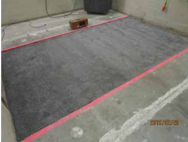
Figure 1 – Specimen mounted in test opening, as viewed from source room (tapping machine removed for test)
