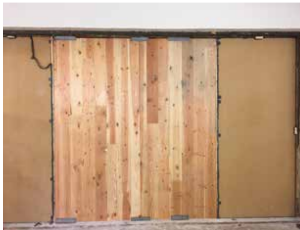
Images this page: the process of receiving the CLT at testing lab, sealing in test opening and assembly build up.
