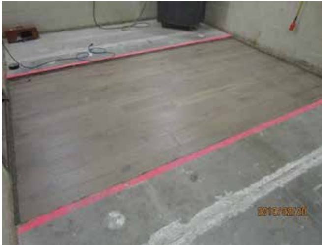
Figure 1 – Specimen mounted in test opening, as viewed from source room
