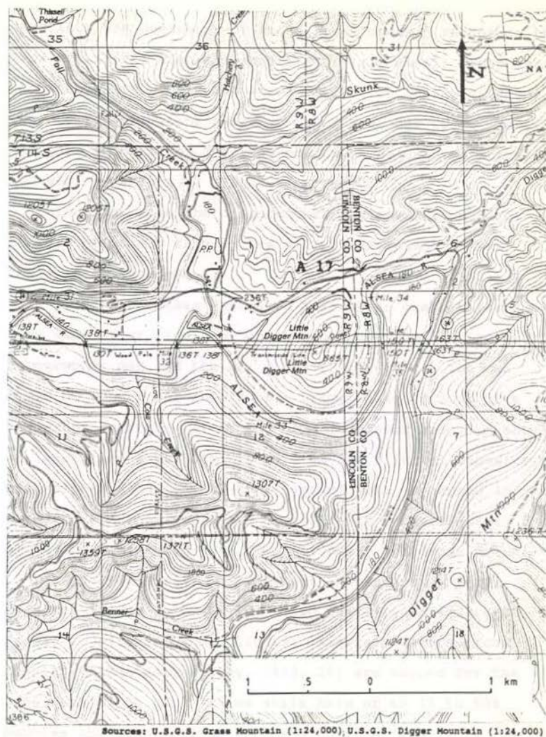
Figure 12. A 17 as an example for a meander cut-off.
