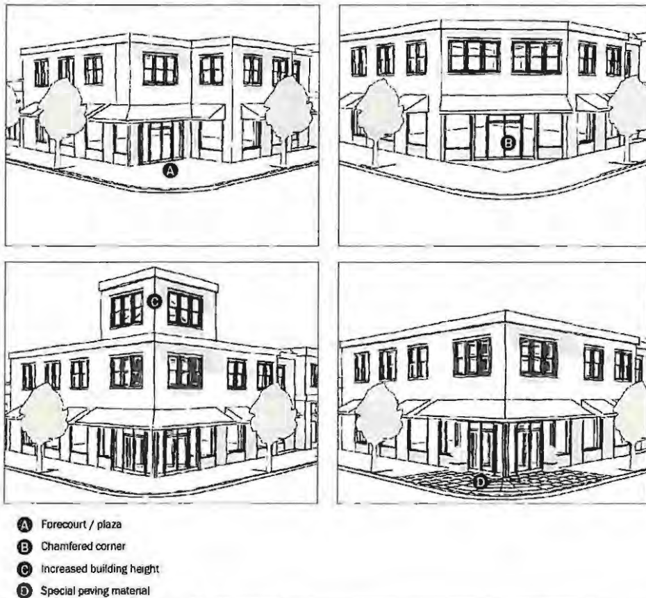
Figure 50.05.004-Q: Building Design at Street Corners
