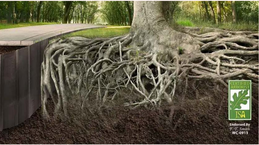
Figure 1.3.11 Root Protection Illustration of vertical root protection, which at least one longterm study found to be the most effective root protection intervention compared to other options, such as horizontal layers of foam and increased aggregate depth (Smiley, 2008, greenindustrytrees.com)
