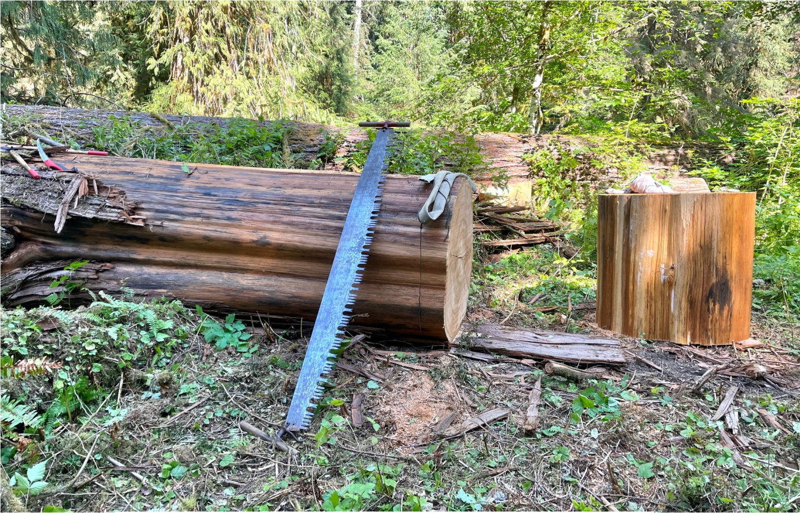
A crosscut saw—affectionately referred to as a ‘misery whip’—used to cut rounds of western red cedar to into roofing shakes, instead of a gas-powered chainsaw. Photo by author, 2022.
