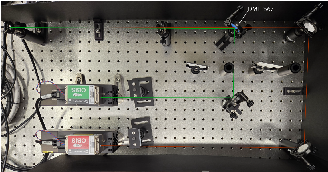
Figure 3.1: Excitation Path. Two OBIS™ lasers are shown (bottom left) with the green and red excitation paths overlain. The two paths combine at the DMLP567 dichroic mirror (top right) and are aligned with two irises (top center and left).
