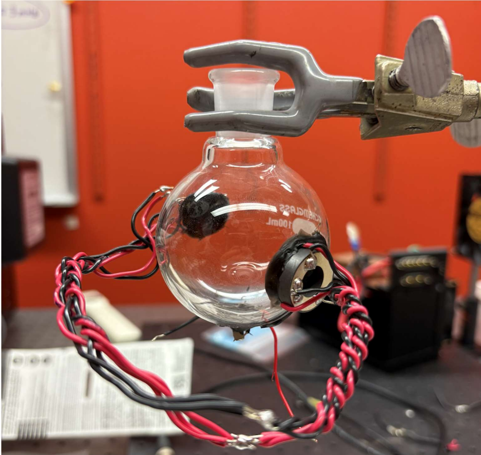
Fig. 8: Opaque neck, small 100 ml spherical flask, two PZTs
