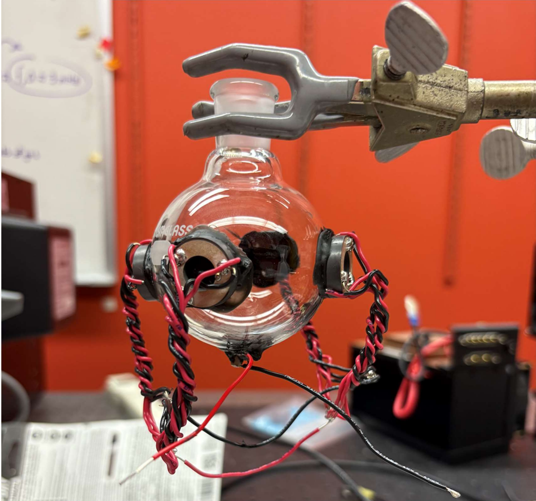
Fig. 9: Opaque neck, small 100 ml spherical flask, four PZTs
