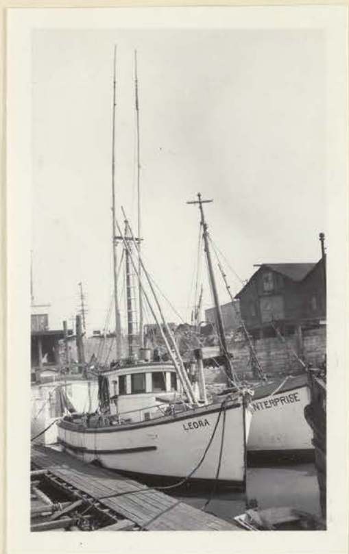
Fig. 1. A typical trolling boat. The arrangement of poles shown here has been most common.
