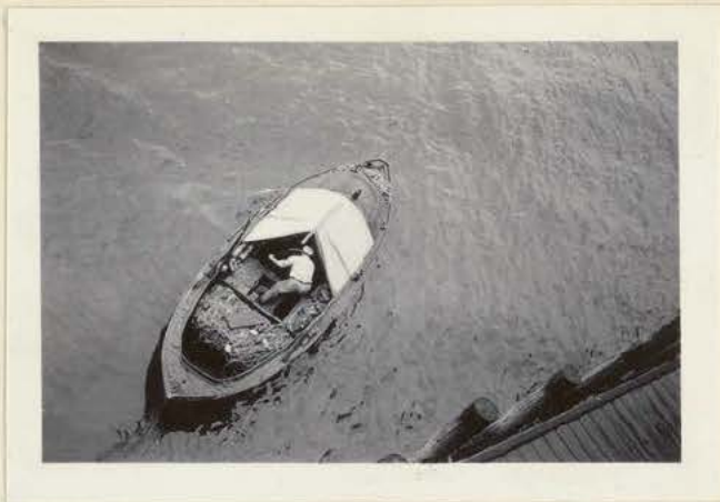
Fig. 14. Columbia River gill-net boat, 1925. The arrangement shown was the one most in favor for the first twenty years or so, following the introduction of power.
