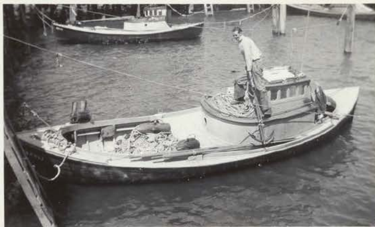
Fig. 15. Columbia River gill-net boat, 1936. The arrangement favored for the last decade is shown. Note that the space for the net has been shifted from the stern to the bow.
