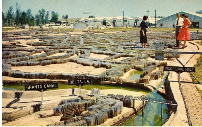
Figure 53. The Mississippi River Basin Model by the U.S. Army Corp of Engineers, physical model. From ElMalvaney, 2010.
