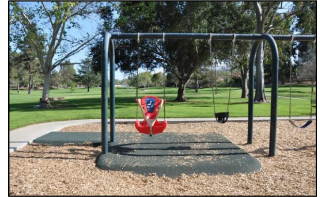
ADA compliant swing installed in Cornona, CA enable both young children and children with special needs to feel the thrill of a ride on a swing and allow their parents to easily and safely take them in and out of the swing via the rubberized surfacing
