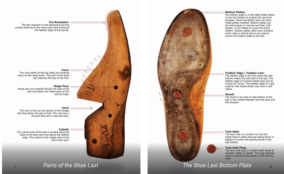
Figure 3: Components of a Footwear Last
