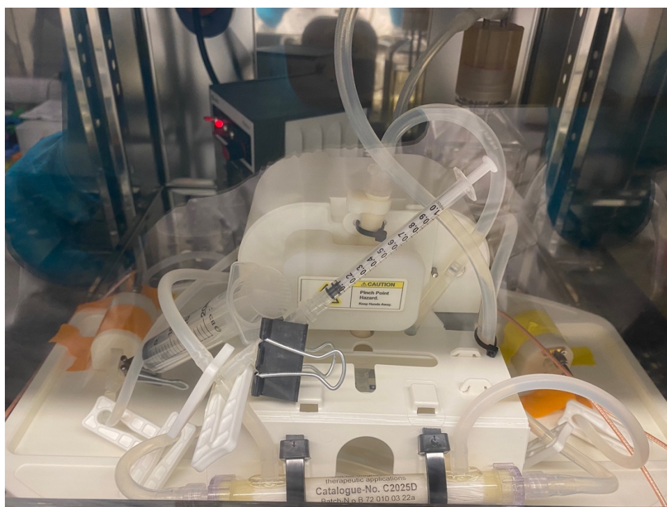
Figure 51. Photograph of the bioreactor system with the integrated magnetoelastic monitoring system inside of the incubator. The auxiliary pump can be seen behind the duet pump in the incubator.
