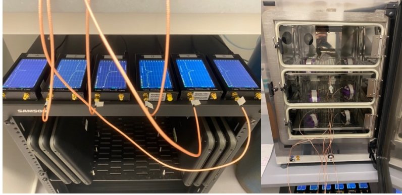
Figure 19. Images of the longitudinal monitoring system deployed in an incubator. 6 computers loaded with custom software are connected to 6 network analyzers via USB to facilitate control and collection of data ( left ). 6 detection solenoids are distributed evenly throughout the incubator to prevent interference between the solenoids ( right ).
