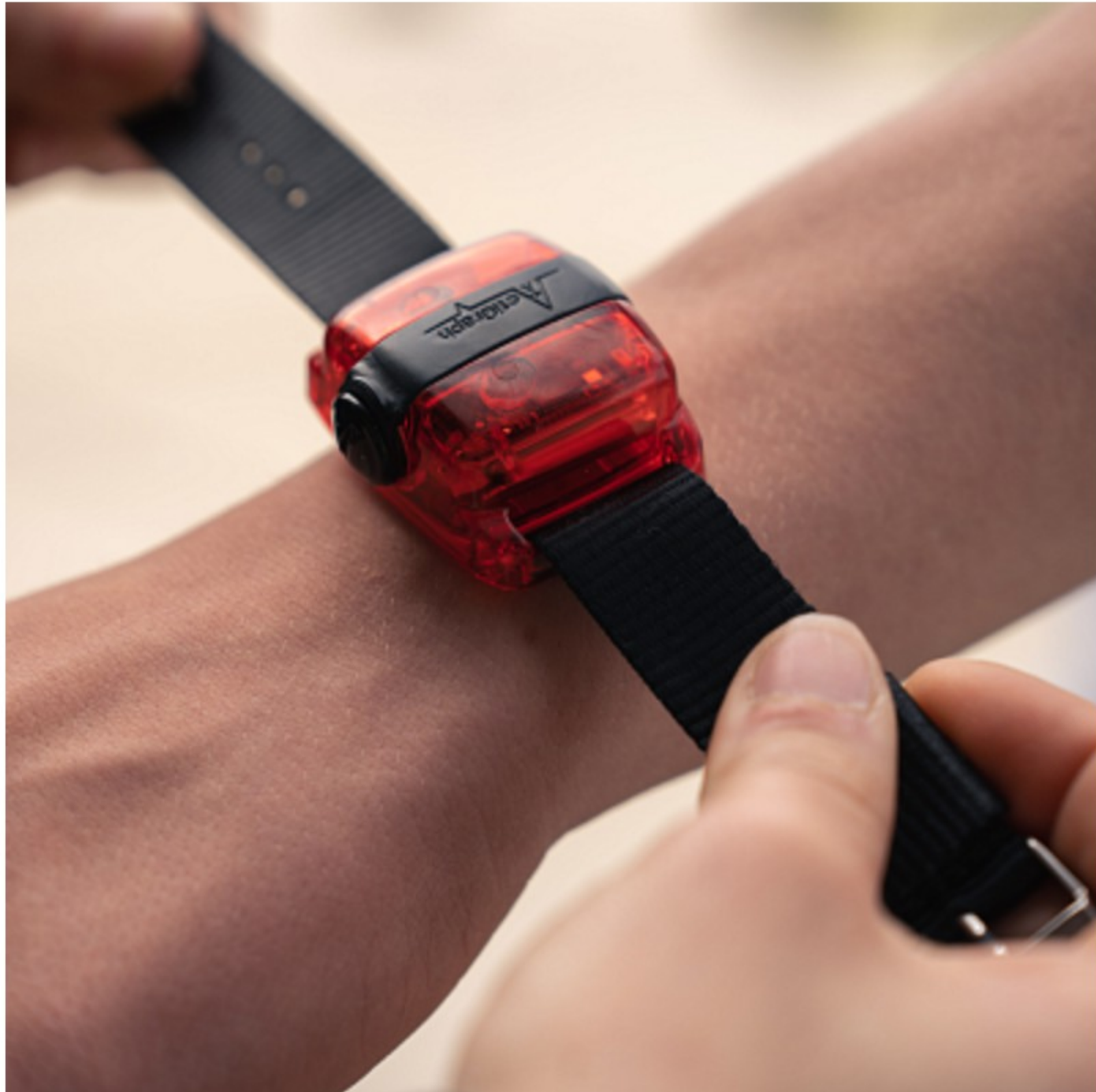
Accelerometers capture sleep patterns and time spent being sedentary or active
