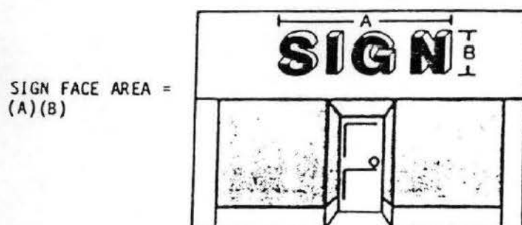
FIGURE 535.2 SIGN FACE MEASUREMENTS
