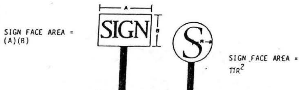
FIGURE 535.1 SIGN FACE MEASUREMENT
