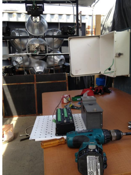
P2. Data acquisition assembly. Solar simulator in the background.
