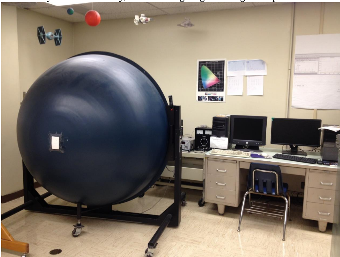
P11. 72" Integrating sphere and spectroradiometers used during the exercise.
