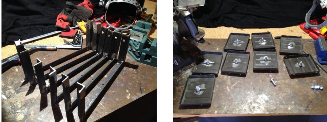
Figure 117: Luminaire Brackets (left) & Pivot Pins (right)
