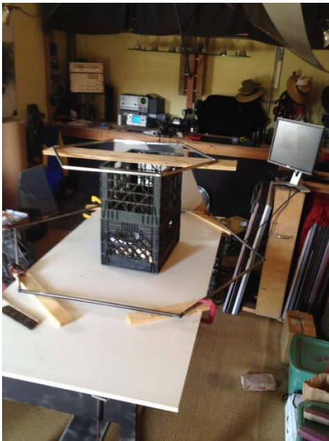
P22. Two hexagonal frames in place to receive the TALBREM mirror.
