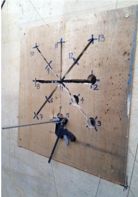
P21. Supplemental guide plate over the back of the Test Plane to guide pyranometer without taking it out at each of the 13 measurement points. Concentrator
