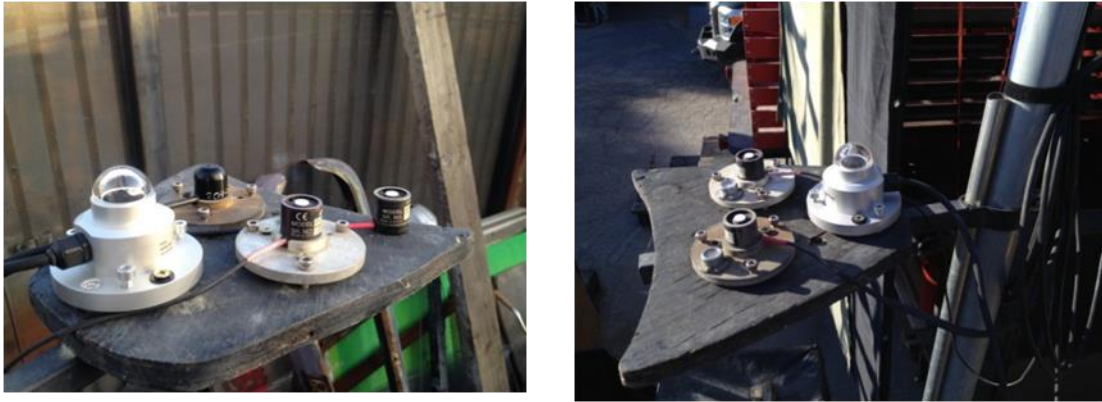
Figure 126: Pyranometer Calibration (Two silicon pyranometers, one hemispherical pyranometer, and one UV sensor)
