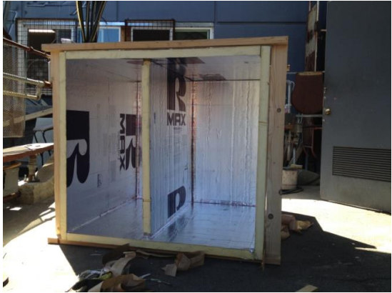
P5. Multiple cell test chamber. When complete the nanowindow will be situated in one chamber and fluids displaced and measured in the second chamber
