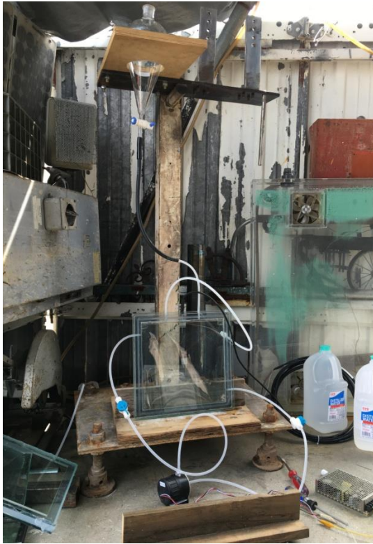
Figure 61: Nanofluid Filling Station Separatory funnel and filling lines leading to Nanowindow prototype (left). Nanowindow prototype (above)
