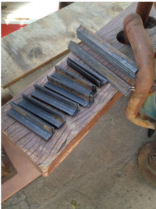
P7. Seven brackets fabricated from 1"x1"x16 gauge steel angles
