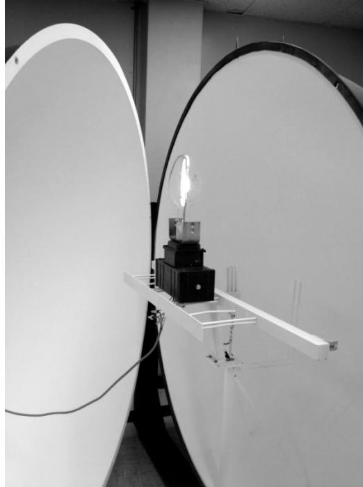
Figure 34: Lighting Lab Integrating Sphere - Metal Arc Placement
