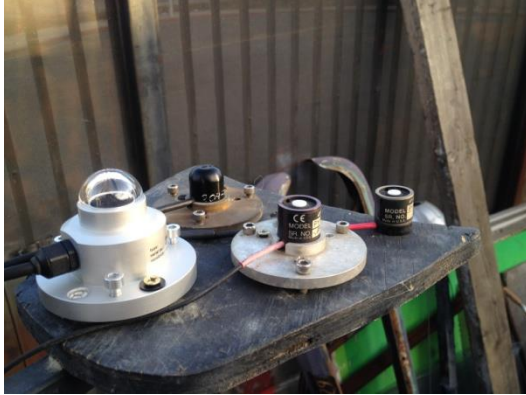
P32. Sensor Hub with two (2) silicon pyranometers and one (1) hemispherical pyranometer and one (1) UV sensors (Left).
