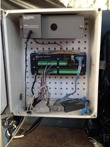
P1. Top to bottom: Power Supply & Battery, CR10X Data Logger, RS32 Interface.
