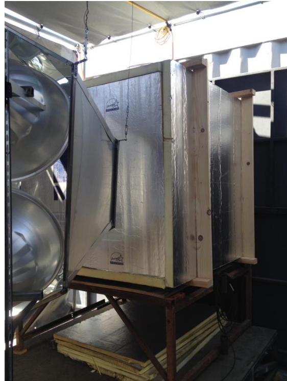
P6. Test chamber situated in front of the solar simulator
