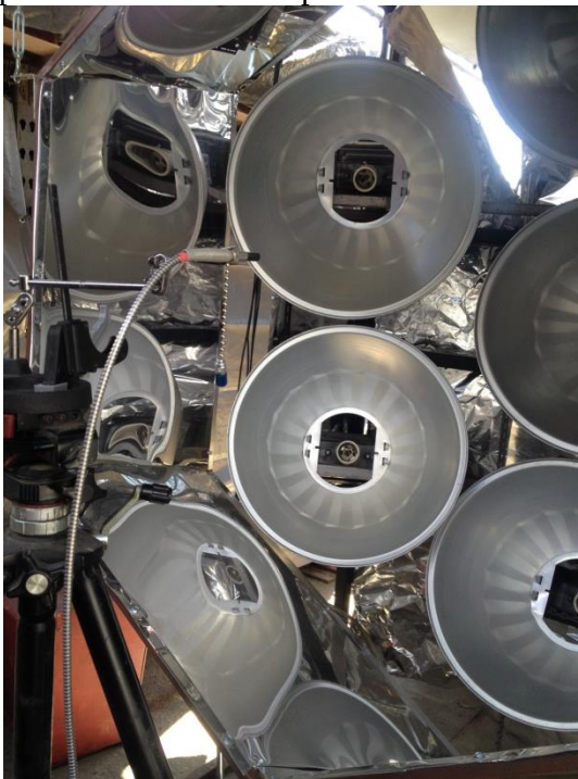
P33. Using the OceanOptics spectroradiometer and fiber optic probe to measure spectral wavelengths of metal arc lamps. Probe attached at the end of a camera tripod.
