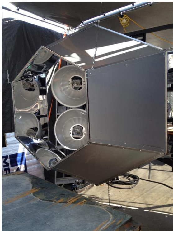
P25. Concentrator suspended from canopy and situated in front of luminaire array.
