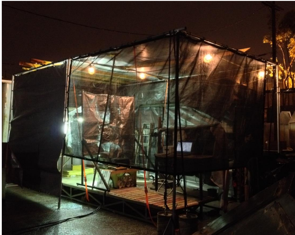
P14. Solar Simulator under canopy
