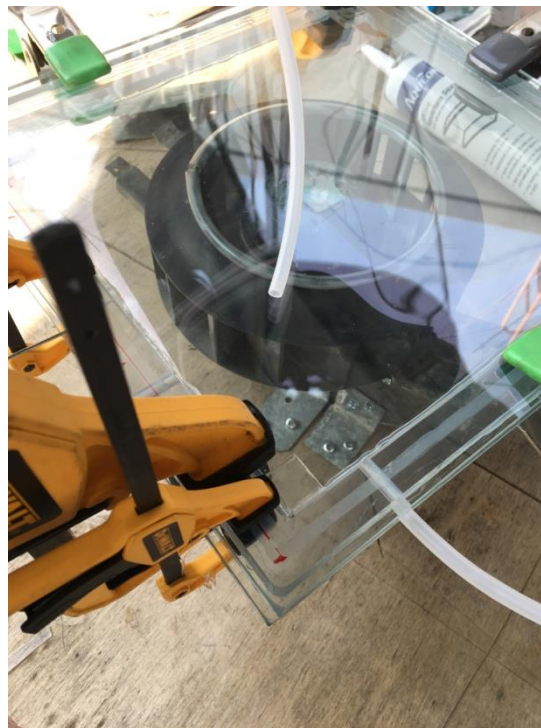
Figure 60: Nanowindow Silicone pressed between glass panes
