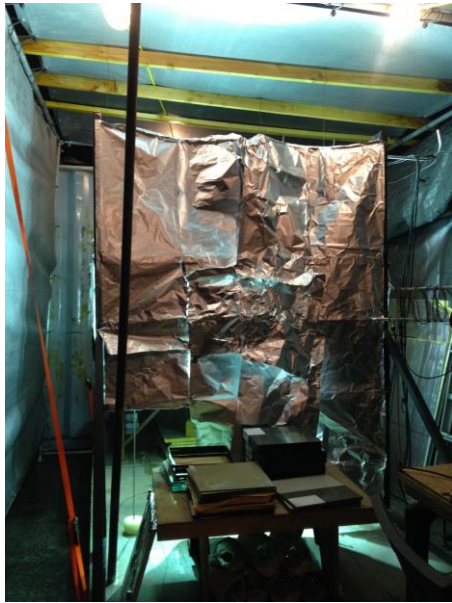
P15. Temporary aluminum foil to block direct line of sight.
