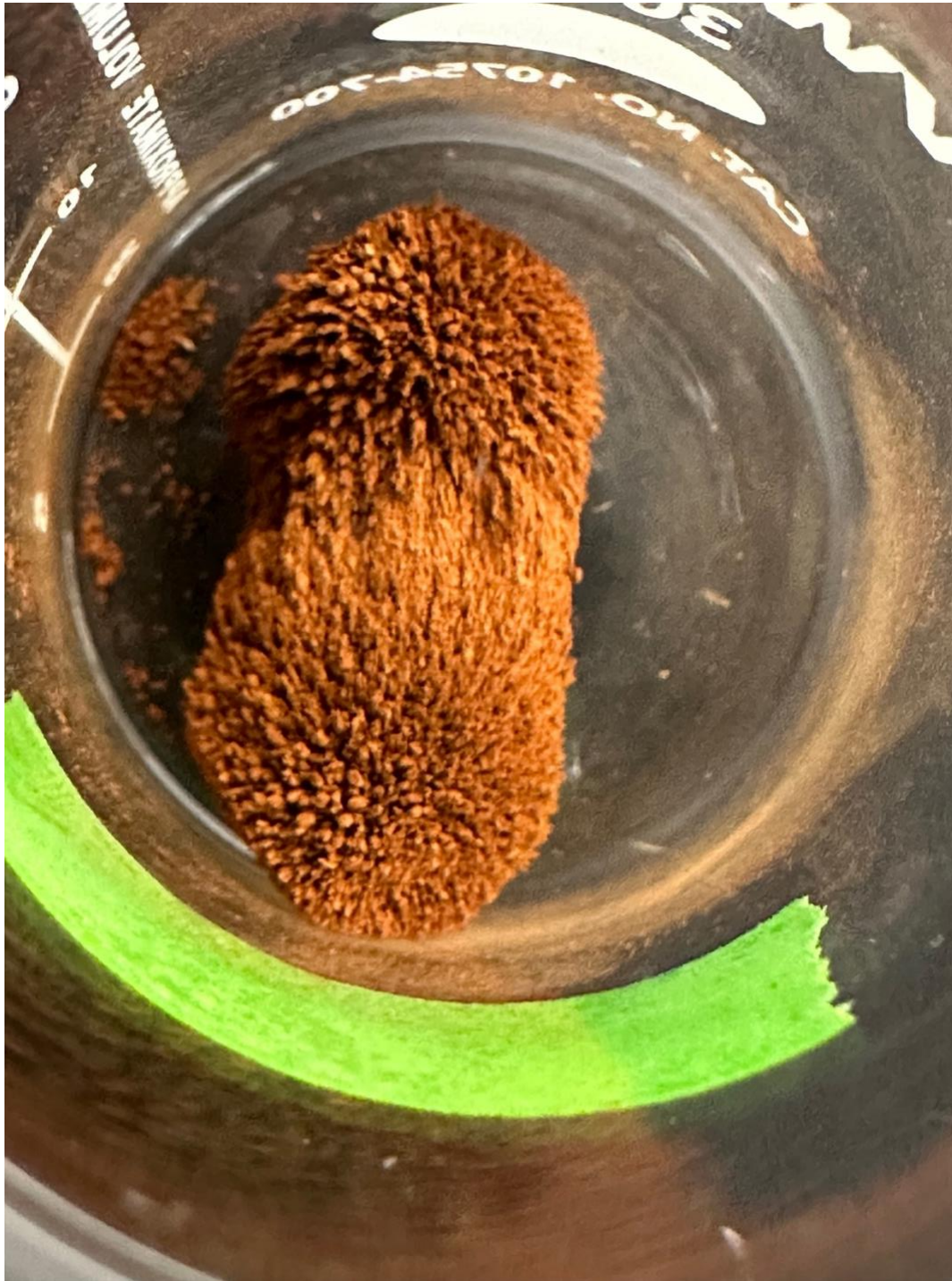
SI Figure 3.13. Burned (800 °C) soils from the summit position demonstrate enhanced magnetism of soils with increased burn intensity (soil is attached to a stir bar).
