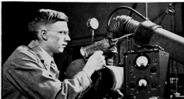
This electronic "sniffer" makes sure that every G-E refrigerator part is leak-proof.
