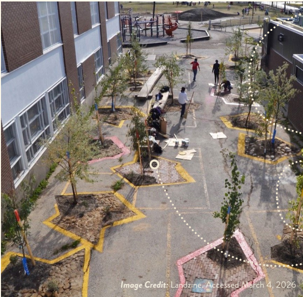
“Folly Forest” by Straub Thurmayr Landscape Architects, Winnipeg, Canada (2013): A low-cost, low-input revegetation of an asphalt schoolyard through depaving and painting uniquely shaped tree-wells.
