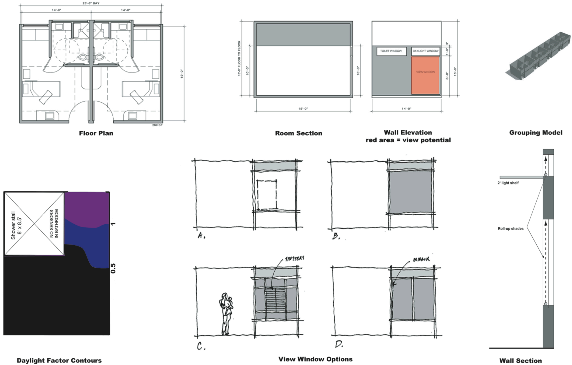
Figure 3 - "Outboard Typical" configuration (Model 1). View window options are: A) Recommended view apertures from Glare calculations, B) Maximum view window, C) Maximum view window with operable shutters or louvers (do diminish backlighting of family members sitting on bench in front of window), D) Recommended view apertures with addition of a mirror placed on wall to increase perceived size of view window.
