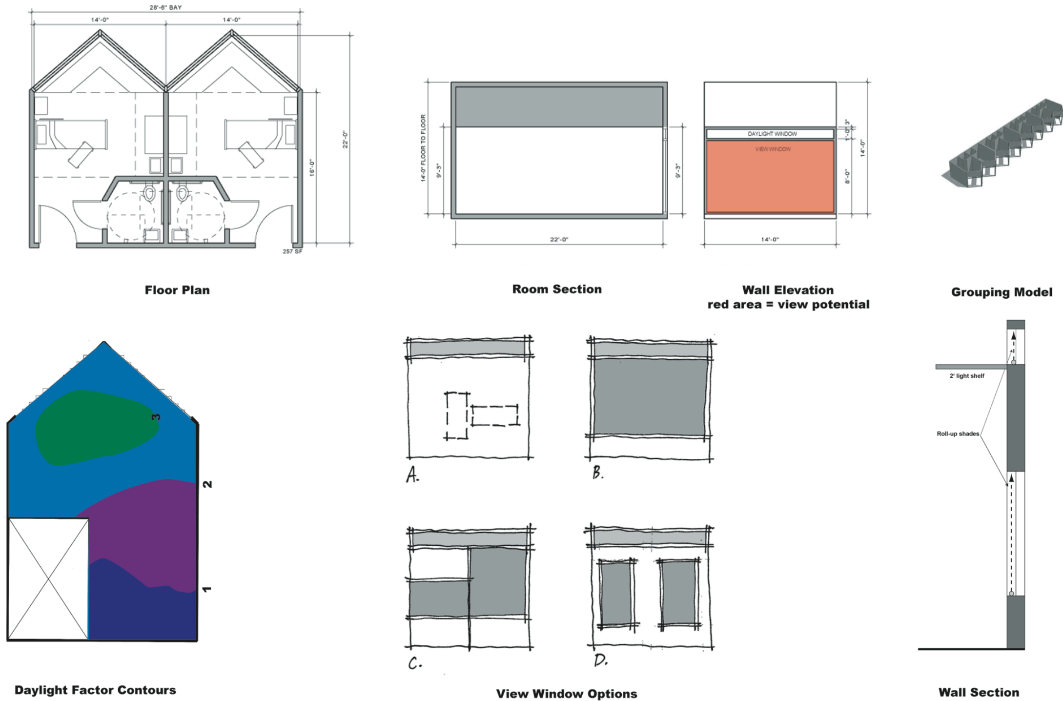
Figure 10 - "Chevron" configuration (Model 12). View window options are: A) Recommended view apertures from Glare calculations, B) Maximum view window, C) Separated patient view and family view windows organized as a composition, D) Separated patient view and family view windows as punched openings.
