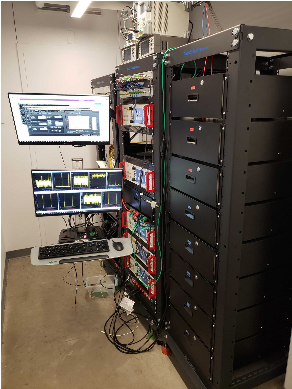
Figure 4.5. The laser racks. Contains our breadboard laser systems used for ionization, cooling, preparation, and readout.
