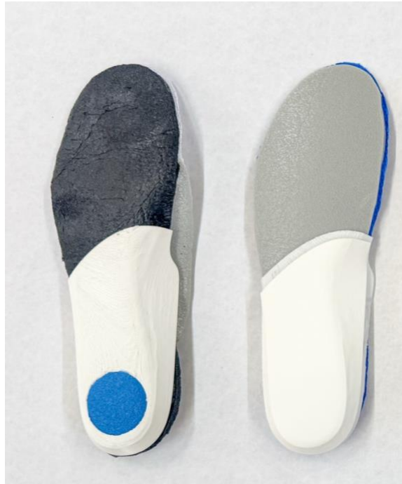
Figure 38: Bottom view of insole #1 (black and blue foam and white PLA sulcus) and insole #2 (grey foam and white PLA stabilizer plate)
