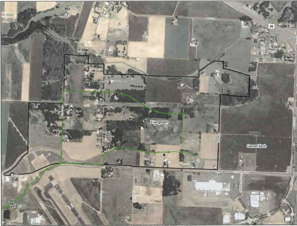
Figure IV.5 Evergreen Concept Planning Area Sanitary Sewer System Conceptual Alternative One Evergreen/Helvetia UGB Concept Plans
