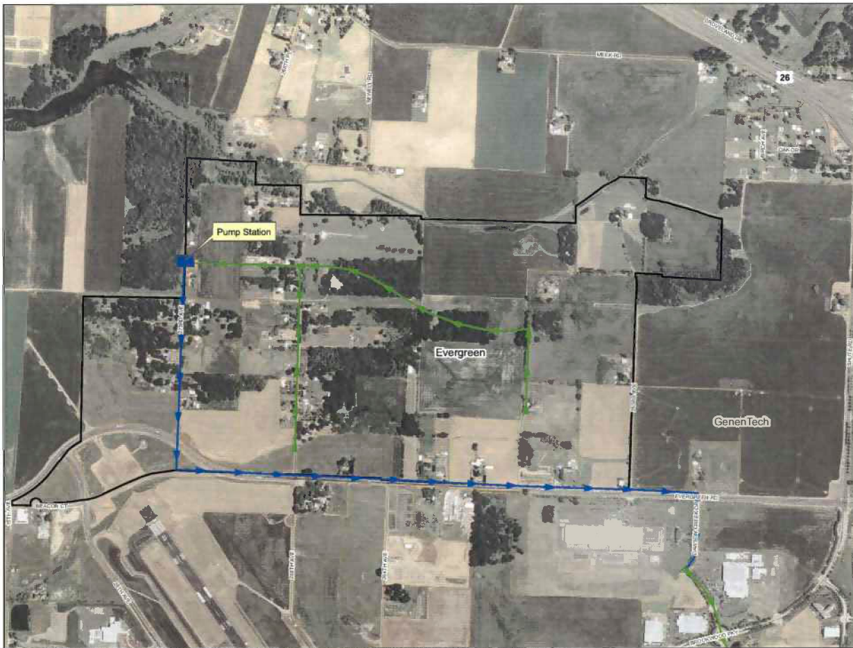
Figure IV.6 Evergreen Concept Planning Area Sanitary Sewer System Conceptual Alternative Two Evergreen/Helvetia UGB Concept Plans
