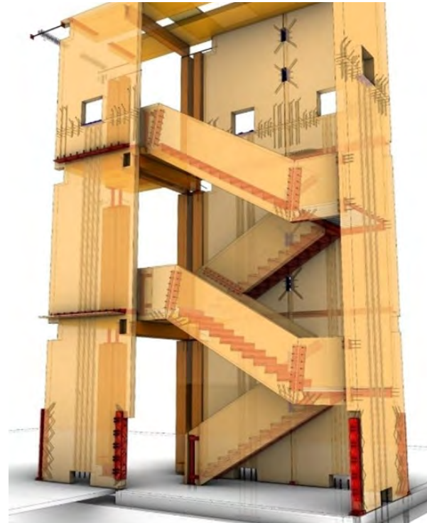
FIGURE 42 | Axonometric Diagram of CLT Rocking Shear Walls (Equilibrium, 2018)
