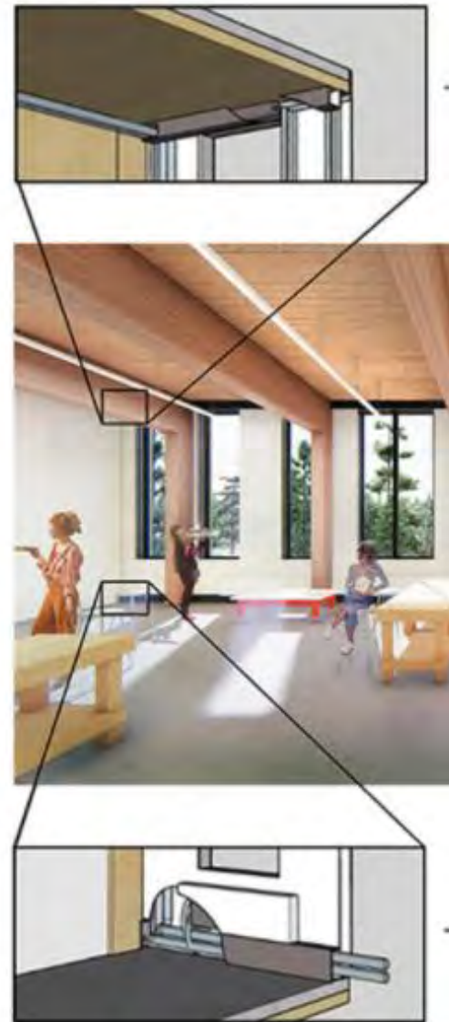
FIGURE 104 | HVAC Units in Exterior Wall. (SRG Partnership, 2017)
