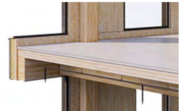
FIGURE 29 | Section Perspective Detail (Michael Green Architecture, 2021)
