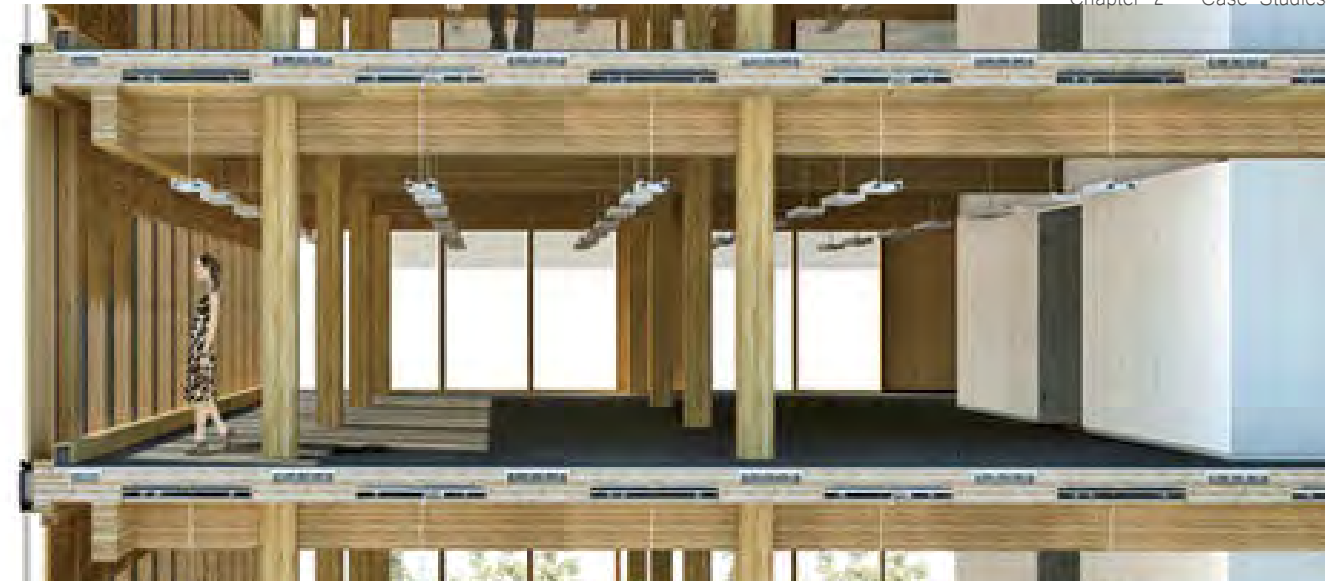
FIGURE 47 | Section Perspective of the WIDC. (Michael Green Architecture, 2015)
