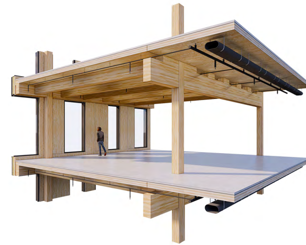
FIGURE 33 | Rendered Section Perspective Detail (Michael Green Architecture, 2021)
