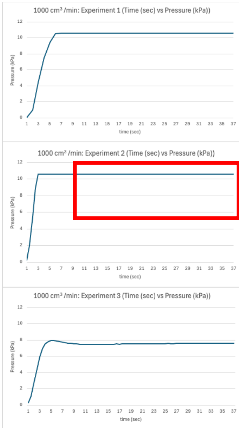
Figure 11: Graphs of 1000 cm 3 /min gas flux pressure measurements. Red box denotes example of pressure stabilization.
