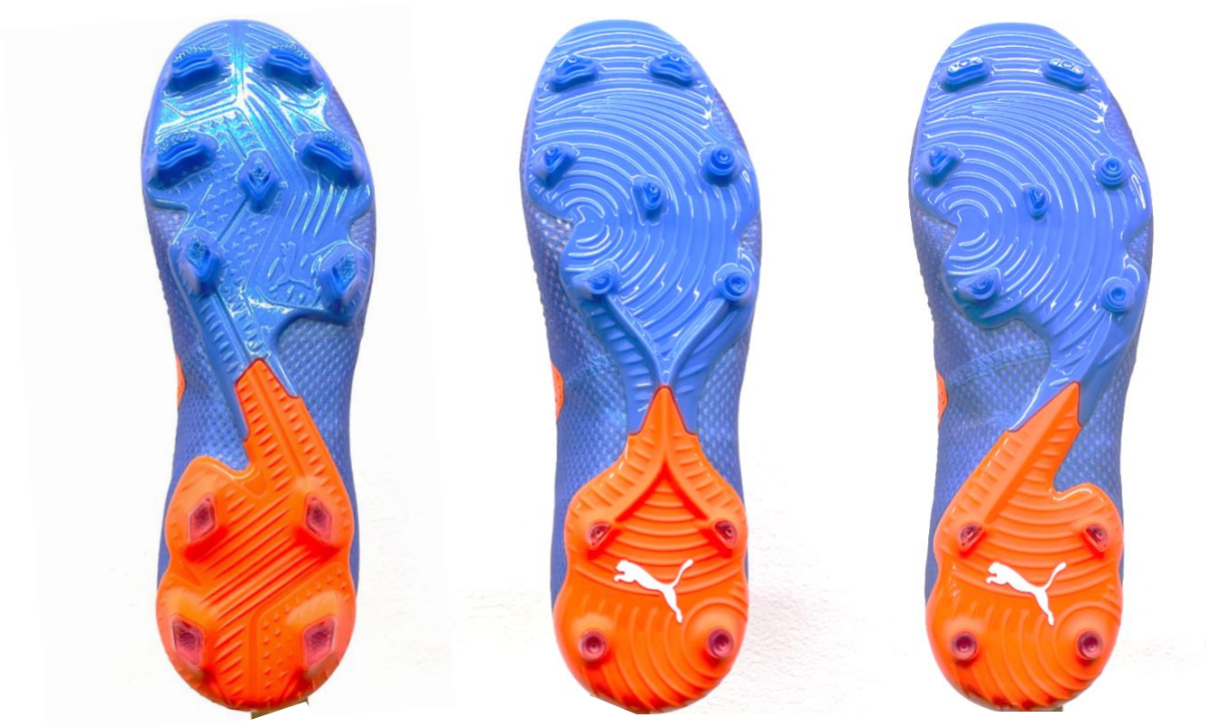
Figure 6.1. Footwear condition outsoles. From left to right: Women's Future Ultimate FG/AG, "Moderate" prototype, "Novel" prototype
