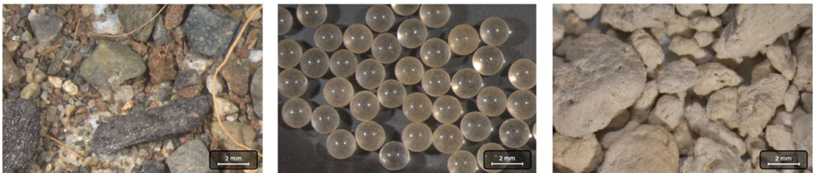
Figure 9. Microscope photos of HPBRM, glass beads, and pumice.
