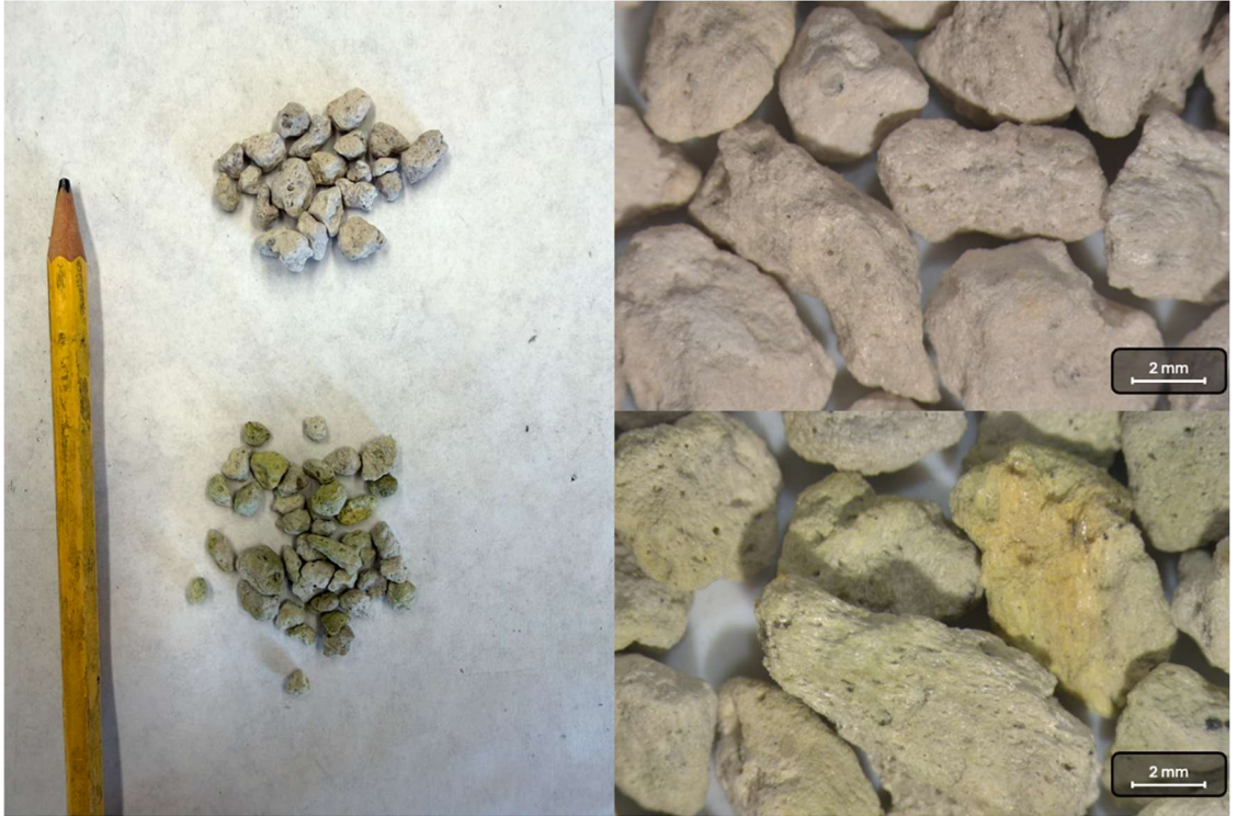
Figure 14. Macroscopic and microscopic images of the 4-8 mm pumice.
