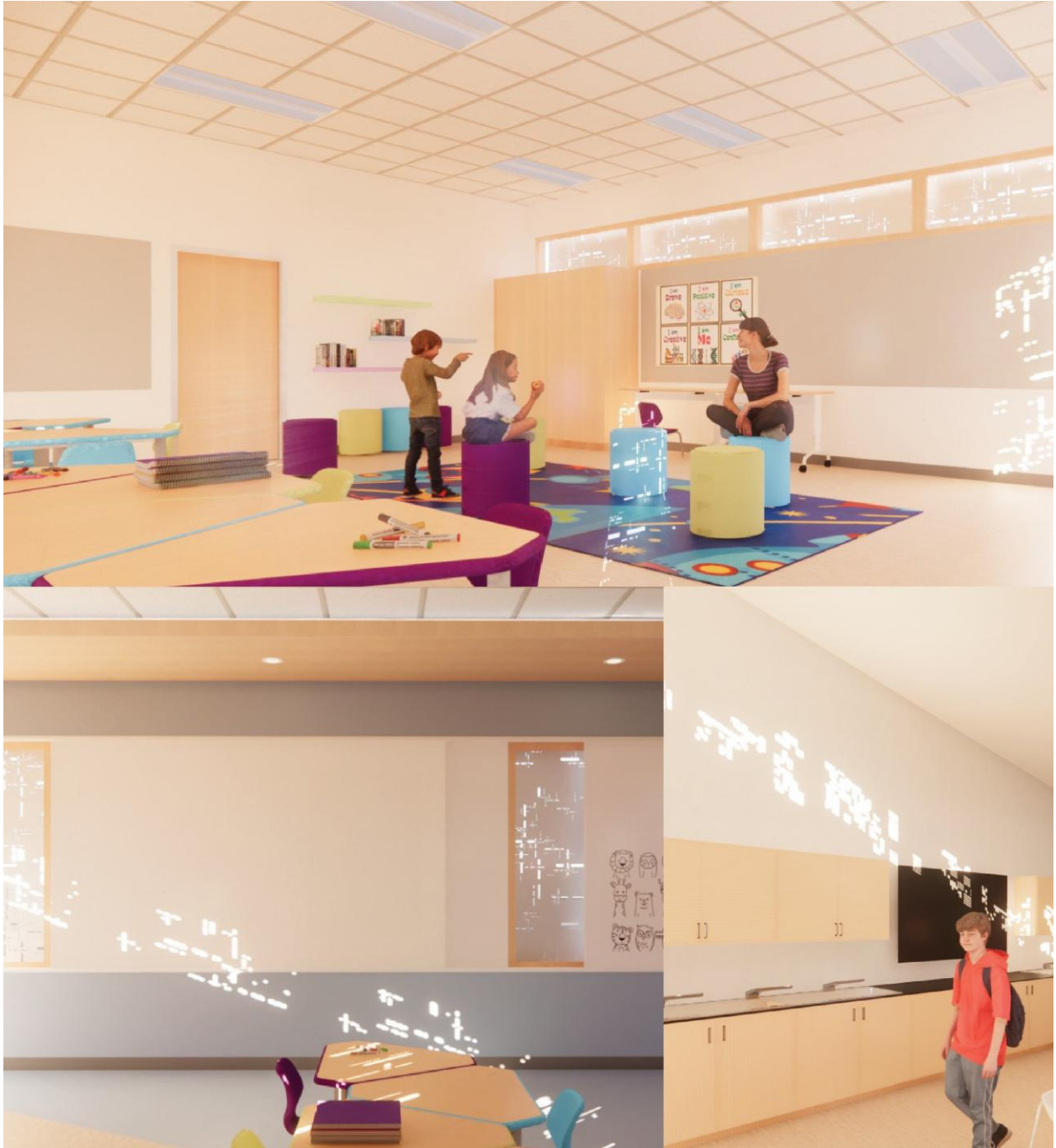
Figure 4.15. Architectural renderings exhibiting the application of perforated solar screens with fractal patterns in a kindergarten and science classroom.
