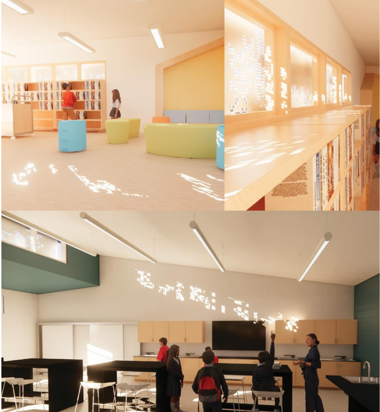
Figure 4.14. Architectural renderings exhibiting the application of perforated solar screens with fractal patterns in a science classroom and library.
