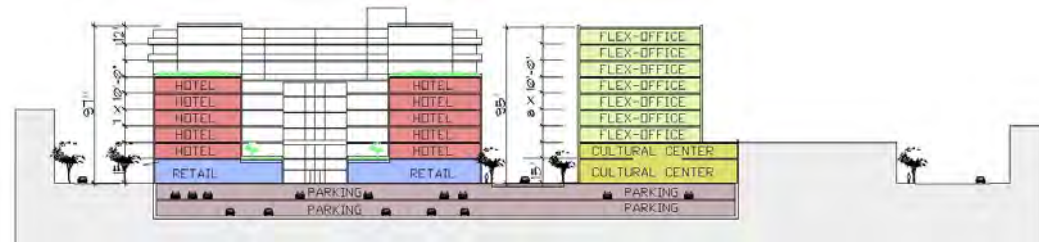
Section A looking north at East Burnside.
