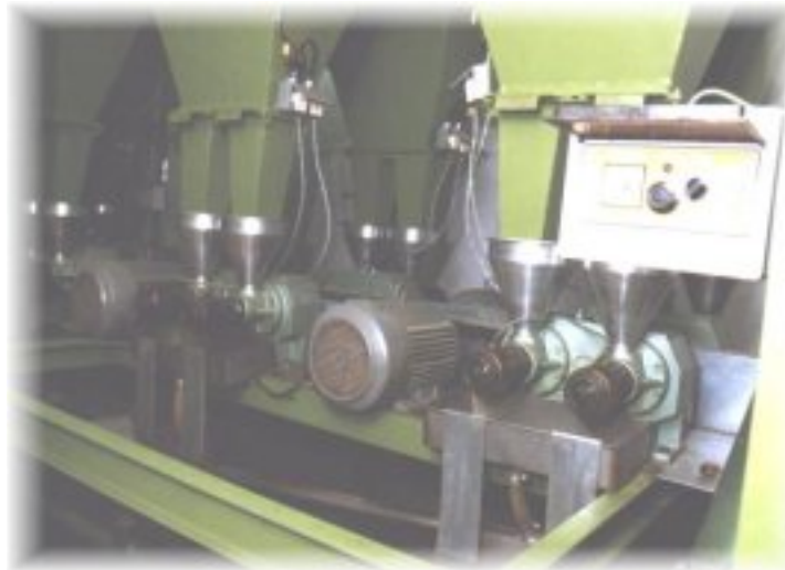
Figure 4. European installation of modular Komet screw presses.
