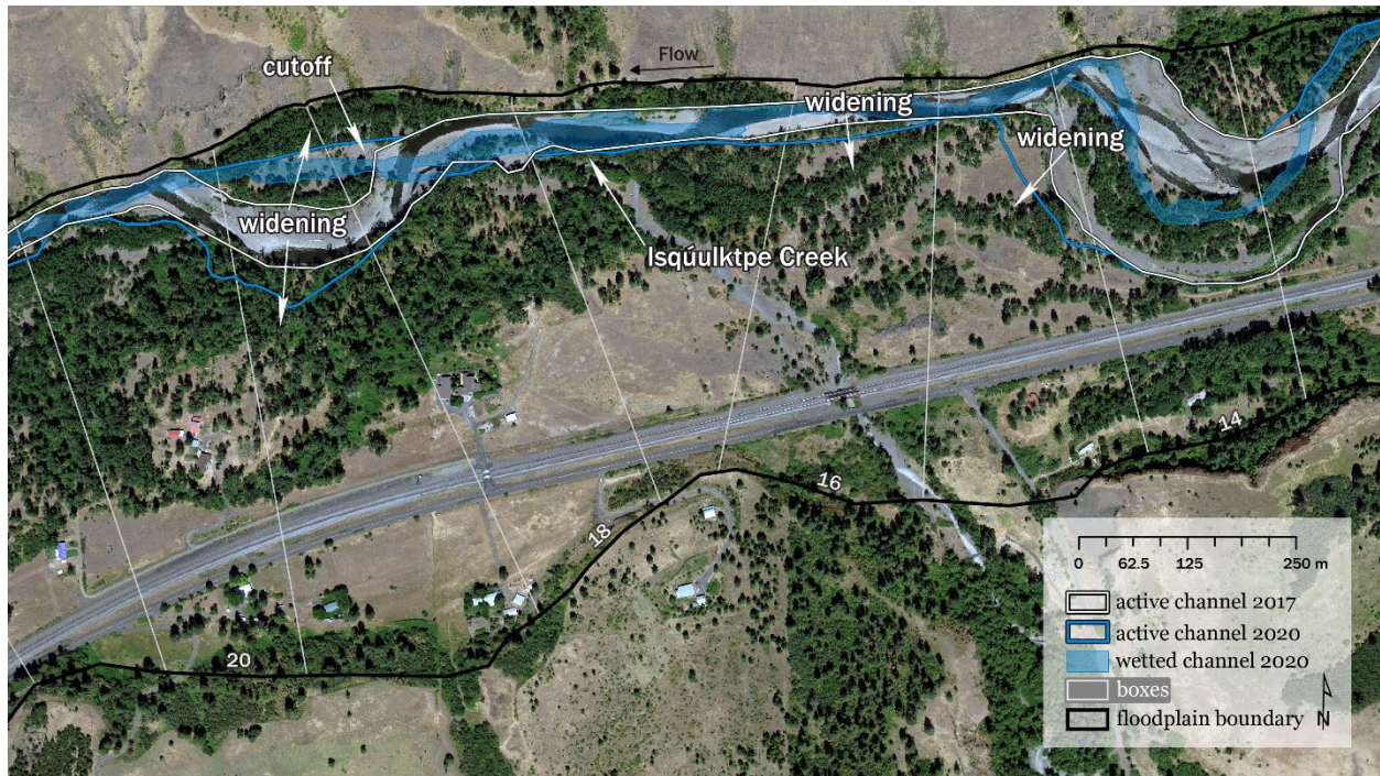
Figure 6. Active channel widening and lateral movement for the 2020 flood (shown on 2017 imagery) in Reach 1 – boxes 14 through 16 and Reach 2 – boxes 17 through 20.
