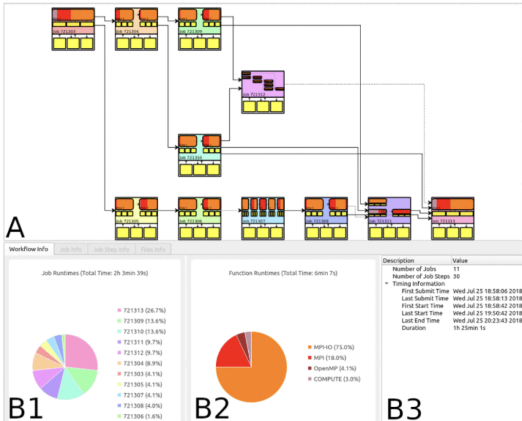
Fig. 11. Top-down performance analysis and visualization methodology: Workflow Visualizer main window consisting of Workflow Graph (A), Job Summary (B1), Function Runtimes (B2), and Info Table (B3) [78].
