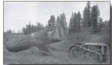
Logging With a Tractor Near Liberty. A 1926 Fordson crawler tractor with one very large log. The tracked version of the Fordson tractor was a factory option available for a short time in 1926–27. It must have been a challenge to go down hill with the set-up above.
