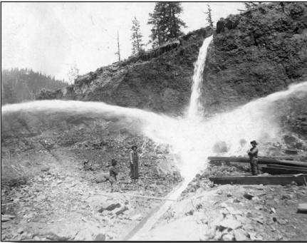
Hydraulic Mining in Liberty in the Early 1900's. High pressure water is being used to wash overburden away to get to placer gold. Hydraulic mining was not successful in Liberty because there was no place for large boulders to go once they were on bedrock and the material above bedrock did not carry much gold.
