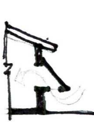
Weather-hood over window for ventilation
