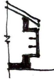
Storage bump-out in lieu of window opening
