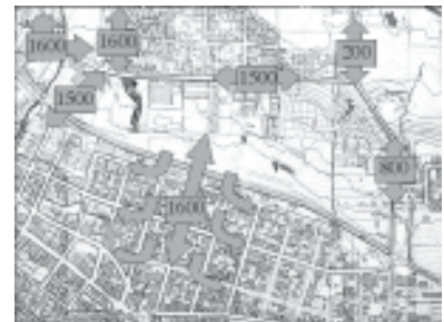
Project daily traffic counts at buildout (with railroad crossing at 4th Street)
