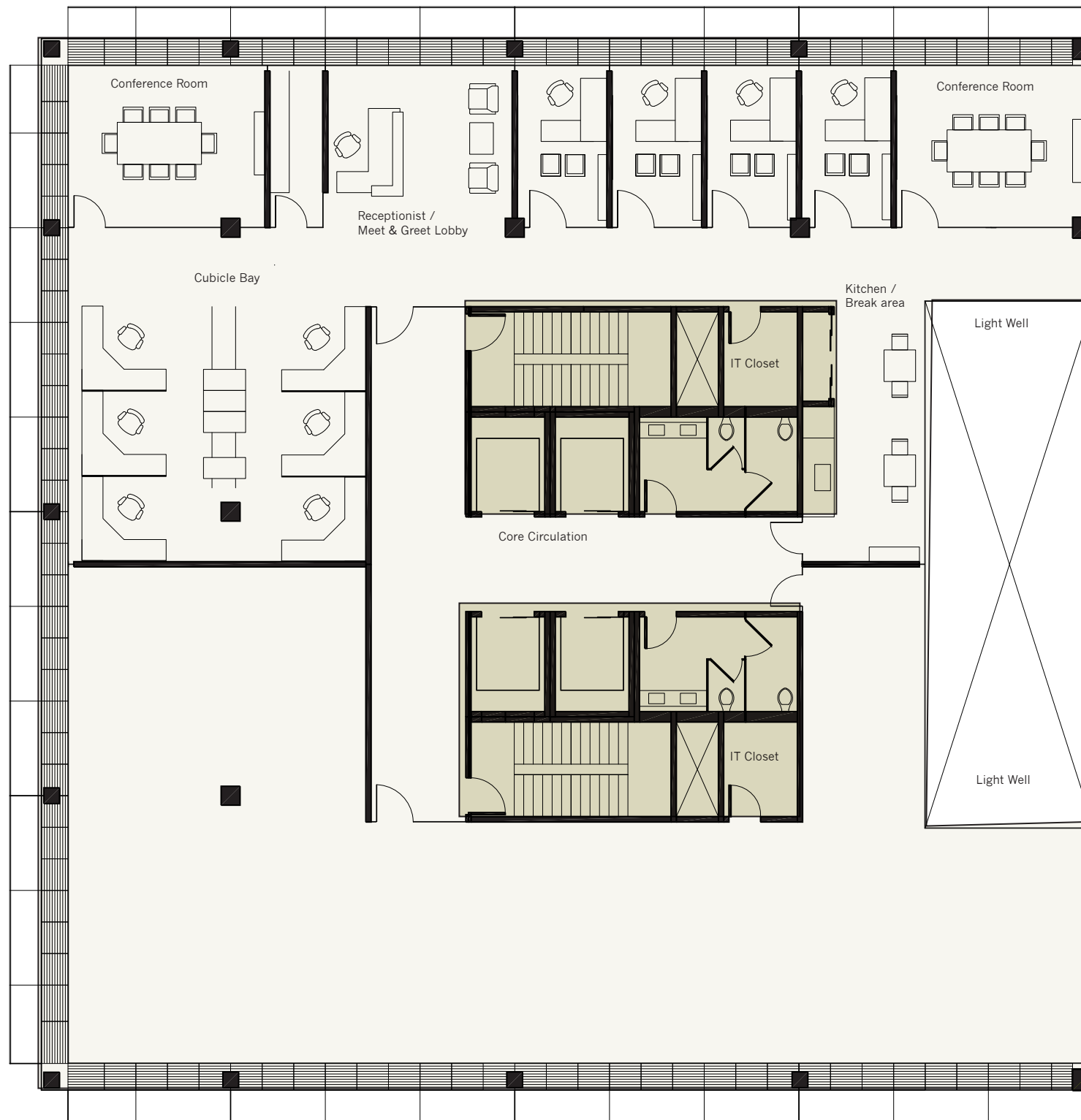
PLAN: FLOOR 8 | TYPICAL HALF OFFICE LAYOUT SCALE: 1/16TH" = 1'
