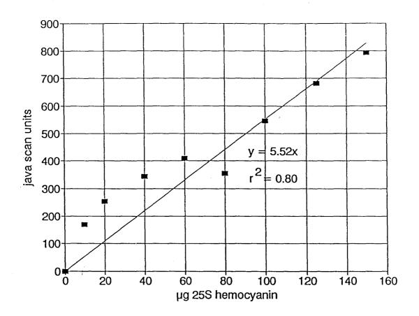
Figure 4. Standard curve relating java scan units to micrograms of 25S hemocyanin.
