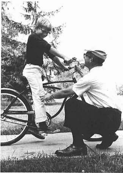
In fitting the bike to the driver, the leg should be fully extended when the driver is seated in the saddle and the pedal is at the bottom of its stroke.
