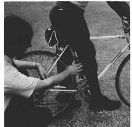
Figure Two. Adjust saddle height with heel on pedal and leg straight.
