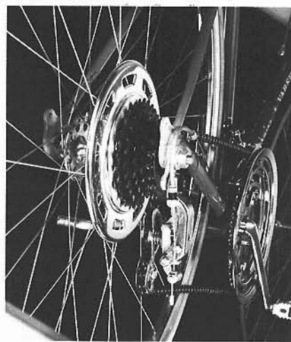
The derailleur "derails" the chain, moving it from one sprocket to another for different gear ratios.
