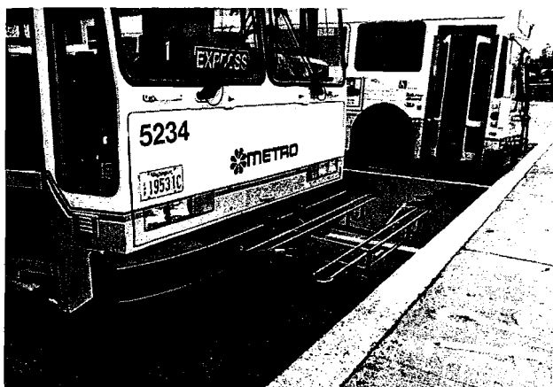
Seattle Metro equipped their buses with a platform style bicycle rack.
