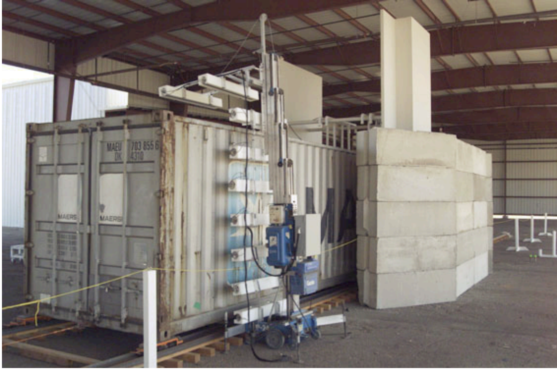
Figure 5. Deployed PPA detector assembly
