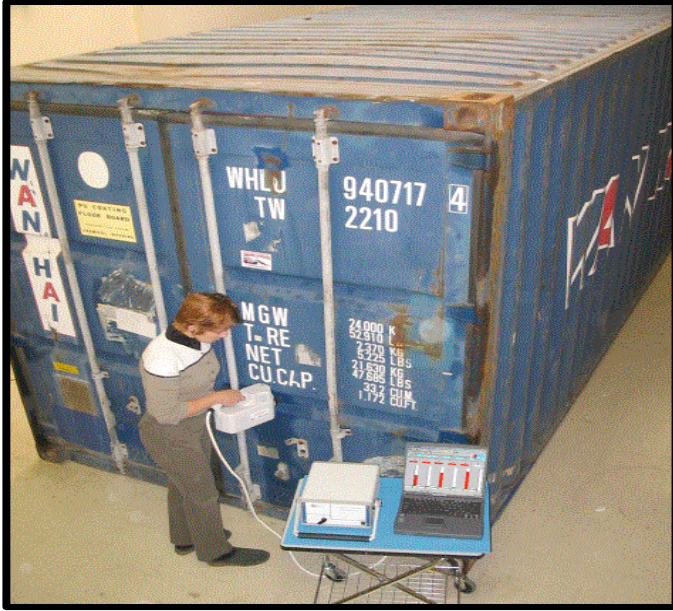
Figure 6. Direct sampling and chemical analysis of odors within a cargo container
