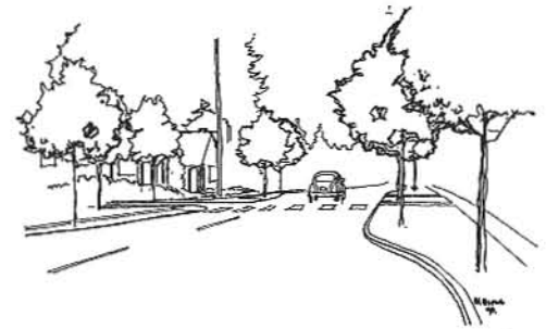
Curb extensions shorten the crossing distance and allow pedestrians to see and be seen before entering the crosswalk.
