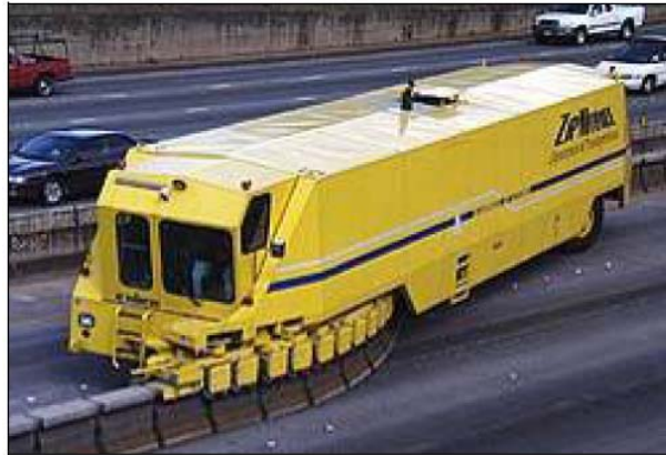
Figure 2: Zipper Machine (Source: FTA Evaluation Report, 2006)
