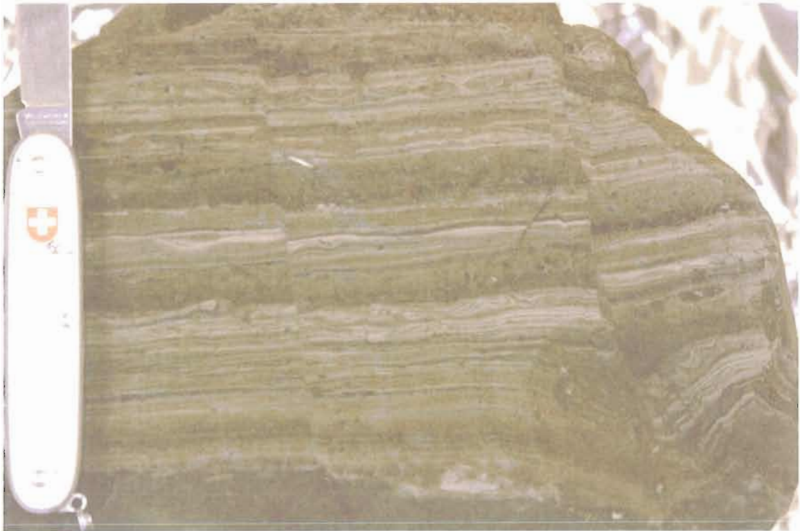
Figure 4. Sample of finely laminated silts. Under a binocular microscope, I picked fine detrital charcoal for ^{14}\text{C} dating. The silts showed extensive faulting and deformation, probably due to post depositional slumping. Knife handle is 94 mm long.
