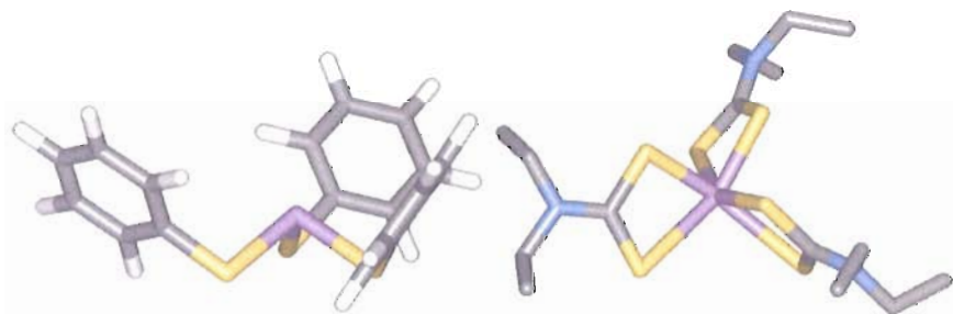
Figure 5 Stereo chemically active lone pair (left) and distorted octahedral (right) crystal structure examples of As(III).
